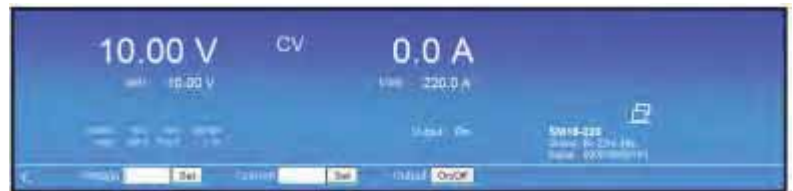
fig. 6 - 1 Front console for setting of the output and monitoring various parameters.
