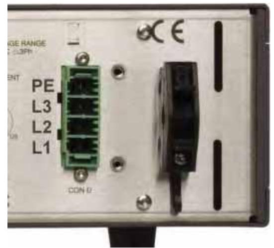
fig. 4 - 2 Insert the included 4-pole header in CON D for the connection of the input power.
