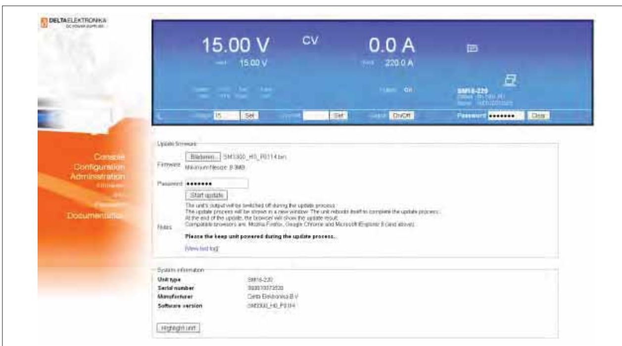
fig. 5 - 3 Via the web interface the downloaded firmware package can be uploaded to the unit.
