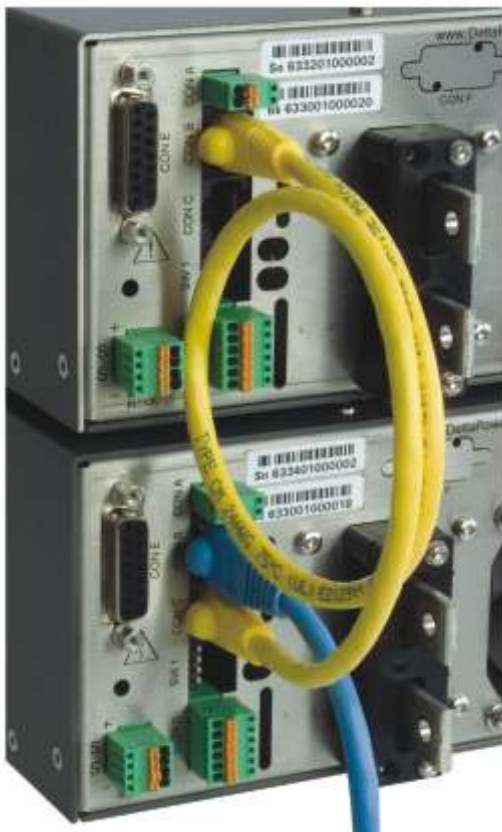
fig. 3 - 21 Use standard UTP cables (RJ45) for Master / Slave operation
