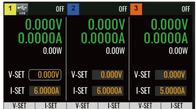
Triple-Channel Meter Interface and Quick Setup Interface
