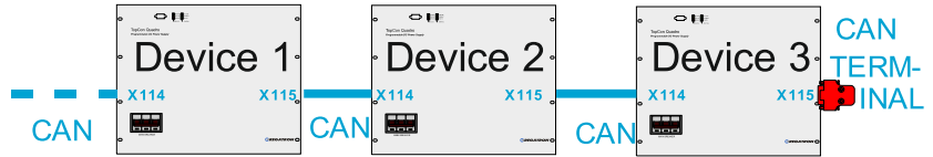
Fig. 1 CANmp bus chain between TopCon devices and termination.
