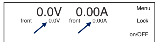
fig 6 - 16 The second line shows the set value for voltage and for source current.
