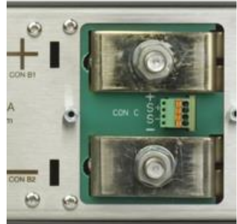
fig 9 - 2 For normal operation links should be connected between S+ and +, and between S- and -.
